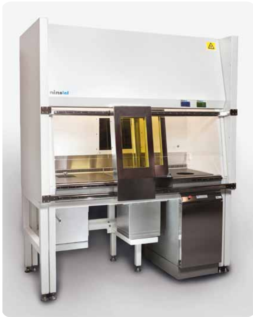
Radiation shielded Microbiological Safety Cabinet combined for both PET and Tc-99 with 50 mm Pb around the cabinet and 30+20 mm Pb equivalent slidably lead glass in front. Integrated generator storage, waste and dose calibrator – all with 50 mm Pb.
