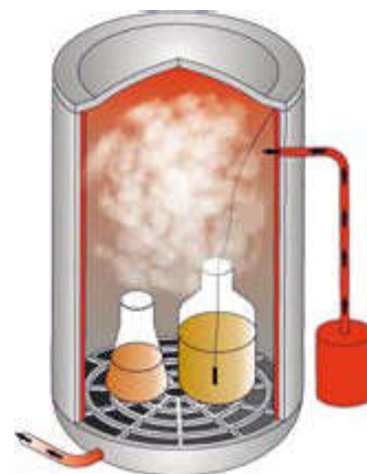
Steam generation using the built-in steam generator
