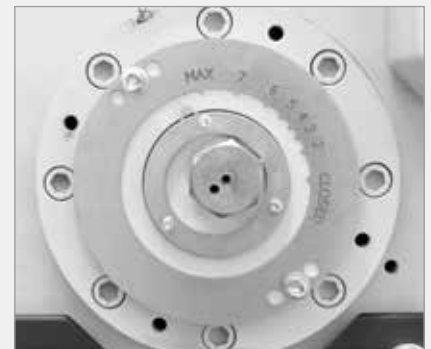
BB 500 XL: Continuous gap width adjustment
