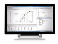
The sieve software EasySieve exceeds manual evaluation in many aspects, due to the fact that it automatically controls the necessary measurement and weighing procedures – from the registration of the weight of the sieve up to the evaluation of the data. It is more simple and more comfortable to use than ever before, and, to put it simple, "easy".
