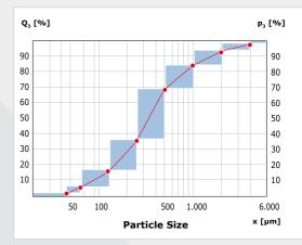
*Fig. 10: Histogram with cumulative distribution curve*
