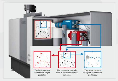
Measurement principle of CAMSIZER P4 with zoom and basic camera
