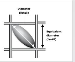
Fig. 16: A lentiform particle can pass the sieve mesh with diagonal orientation (diameter > equivalent diameter)
