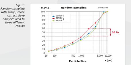
Therefore, it is essential that sampling is carried out with utmost care. A basic requirement for reproducible sieve analysis is the extraction of a **representative sub-sample** from the bulk. Representative means that the properties of the sub-sample, in this case the particle size distribution, have to be identical with those of the bulk.
