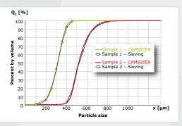
Comparison of CAMSIZER results with sieve analysis for two different samples
