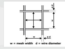
*Fig. 20: Schematic of a sieve mesh*
