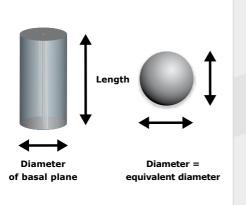
Fig. 15: Comparison between stick and sphere (diameter of basal plane or diameter of sphere = equivalent diameter)
