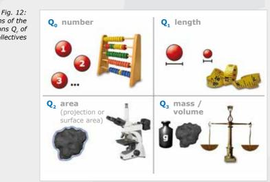
Fig. 12: Definitions of the quantifications Q<sub>r</sub> of particle collectives
