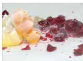
Material embrittled with liquid nitrogen
