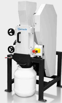
**The Jaw Crusher BB 250 is specifically designed for accepting large feed sizes up to 120 x 90 mm. The gap width can be set stepless from 0-30 mm. Depending on the sample material, particle sizes down to 2 mm can be obtained, resulting in a crushing ratio of 45. A throughput of up to 300 kg/h is possible with the BB 250.**
