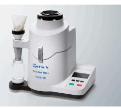
The cyclone mill TWISTER is specially designed for the processing of foods and feeds for subsequent NIR analysis. The optimized form of rotor and grinding chamber generates an air jet which carries the ground sample through the **integrated cyclone** into the sample bottle. The air jet prevents the material from heating up, thus **preserving the moisture content**.
