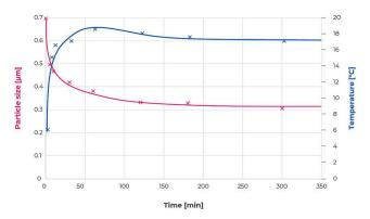
Particle size and temperature development for  ${\rm TiO_2}$  in a wet grinding process with 30 Hz and 2 x 125 ml jars
