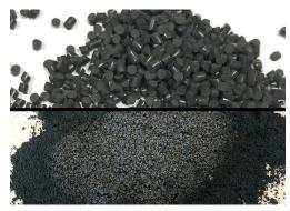
Fast milling of black Flurocarbon rubber (FKM) by embrittling the sample in two 125 ml jars at –100  $^{\circ}$ C.
