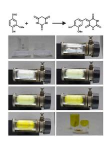
Time course of the Knoevenagel reaction between vanillin and barbituric acid under mechanochemical conditions using 2x10mm zirconium oxide grinding balls in 19 ml PMMA grinding jar at 30 Hz. Reaction running over 30 minutes with visible progress indicated by color change.
