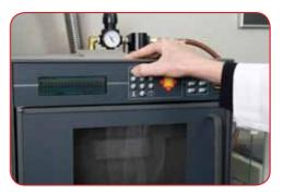
Select the ashing program for your sample using the keypad on the Phoenix Ashing Furnace
