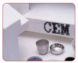
Use any crucible that may be used in a conventional muffle furnace including platinum.
