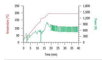
iWave sensors allow for fine power control, as shown in this graph. Temperatures can then be held tighter and digestions are more reproducible.
