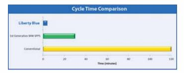
The 4-minute cycle time of the Liberty Blue System is not limited to easily synthesized peptides. These methods can be used to routinely synthesize a wide range of peptides. Using the standard Liberty Blue methods, A-beta 1-42 was prepared in less than **4 hours** in 68% crude purity.
