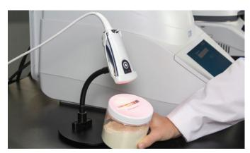
A barcode scanner is included with each system. This enables you to automatically import customer codes into sample ID's.
