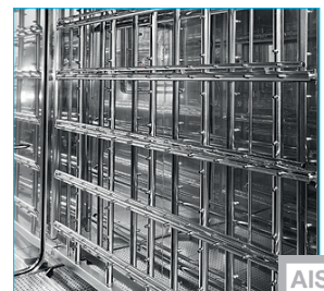
Washing chamber made of s.s. AISI 316L
