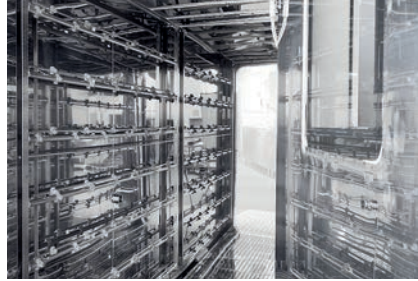
Horizontally mounted oscillating arms to wide spray pattern.
