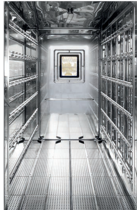
Multiple horizontally and vertically mounted oscillating arms equipped with stainless steel spraying nozzles.
