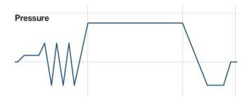
For efficient, high-volume sterilization of heat-sensitive materials (plastic, rubber products and macrolon cages). Pre-vacuum cycle utilizes a mechanical air evacuation system.
