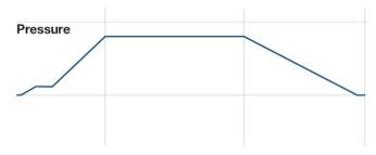
For the sterilization of liquids and media in vented borosilicate glass or metal containers. Liquid cycle utilizes the optimal solution cooling feature, during exhaust (cooling) phase, to control the exhaust rate.
