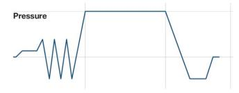
For efficient, high-volume sterilization of porous, heatand moisture-stable materials (utensils, glassware, textiles). Pre-vacuum cycle utilizes a mechanical air evacuation system.
