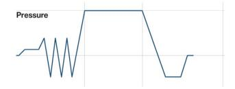
This cycle is used to verify the effectiveness of the steam penetration and air removal for the sterilizers provided with a vacuum pump.
