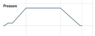
For the sterilization of heat- and moisturestable goods and decontamination of bagged non-biohazardous laboratory wastes. Gravity cycle utilizes the gravity airdisplacement principle.
