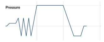
This cycle is used to verify the effectiveness of the steam penetration and air removal for the sterilizers provided with a vacuum pump.
