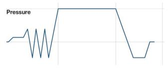
For efficient, high-volume sterilization of porous, heatand moisture-stable materials (utensils, glassware, textiles). Pre-vacuum cycle utilizes a mechanical air evacuation system.
