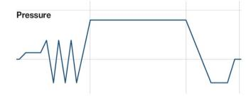
For efficient, high-volume sterilization of heat-sensitive materials (plastic, rubber products and macrolon cages). Pre-vacuum cycle utilizes a mechanical air evacuation system.
