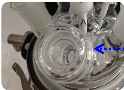
Filling port for solid/liquid feed
