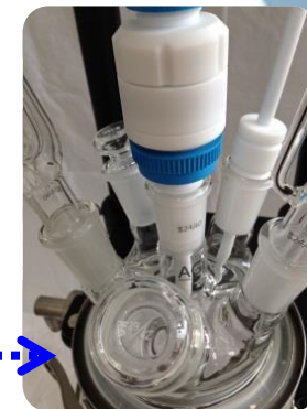
PTFE Mechanical Seal Bearing
