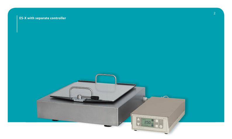
The ES-X is a specially designed shaker with a separate controller. It is ideal for use in existing incubators or temperature controlled rooms as the shaking unit with its stainless steel casing can be placed in areas of high temperature (up to 80°C) and humidity (up to 95% rH).
