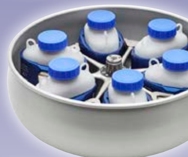
6 x 2000 mL rotor 4,700 rpm 7,187 x g
