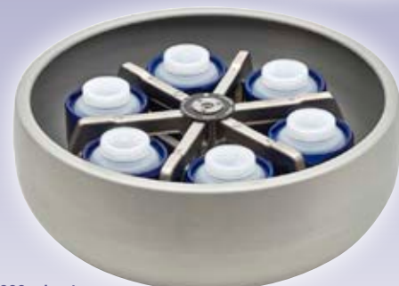
6 x 1000 mL rotor 5,400 rpm 8,500 x g
