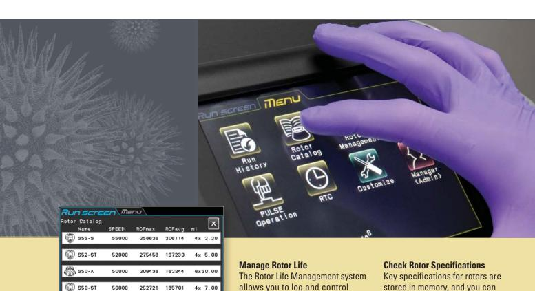
The Rotor Life Management system allows you to log and control individual rotor usage by tracking the number of rotor runs and total spin hours.
