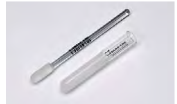
Homogeniser with overflow flare, without lip and glass pestle, cylindrical
