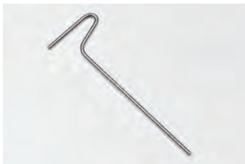
Inoculating hook made of stainless steel (Drigalski-hook)
