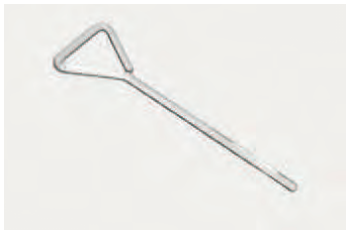
Inoculating hook made of glass (Drigalski-hook)
