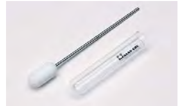
Homogeniser as centrifuge tube with PTFE pestle, cylindrical
