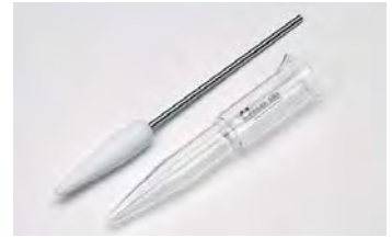
Homogeniser with overflow flare with lip and PTFE pestle, tapered
