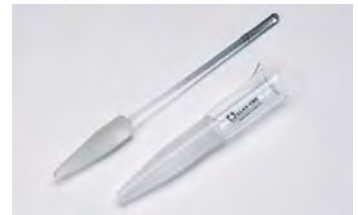
Homogeniser with overflow flare with lip and glass pestle, tapered
