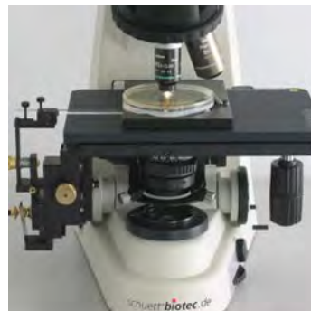
Mechanical stage with micromanipulator *Image similar
