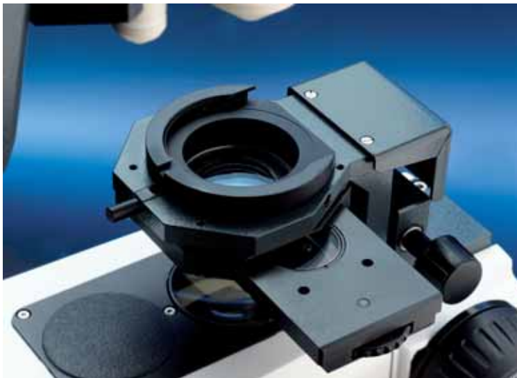
The polarizer slider has two positions, one for visible and one for infrared light. The contrast adjustment according to S enarmont is performed by turning a knob to the right or left.
