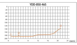
1 Precooling stage when freezer filled to high level
