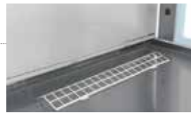
Debris grid catches debris such as paper scrap to damage negative pressure zone.
