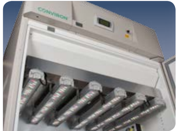
A1000 Chamber with Valoya NS1 LED fixtures
