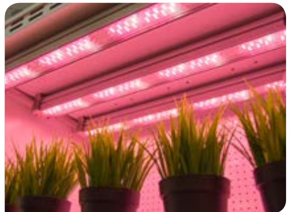
A1000 Chamber with Valoya LED fixtures
