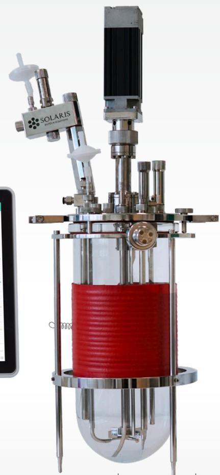
Powerful/ Accurate **brushless motor**, from 1 to 2000 RPM.
