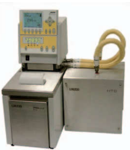
HTC angeschlossen an Proline P 5 C HTC connected to Proline P 5 C
