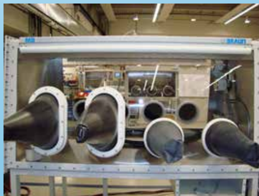
Gloveport feedthrough, round and oval
