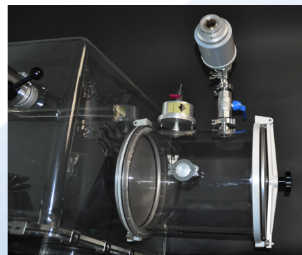
Top view of the purge antechamber
