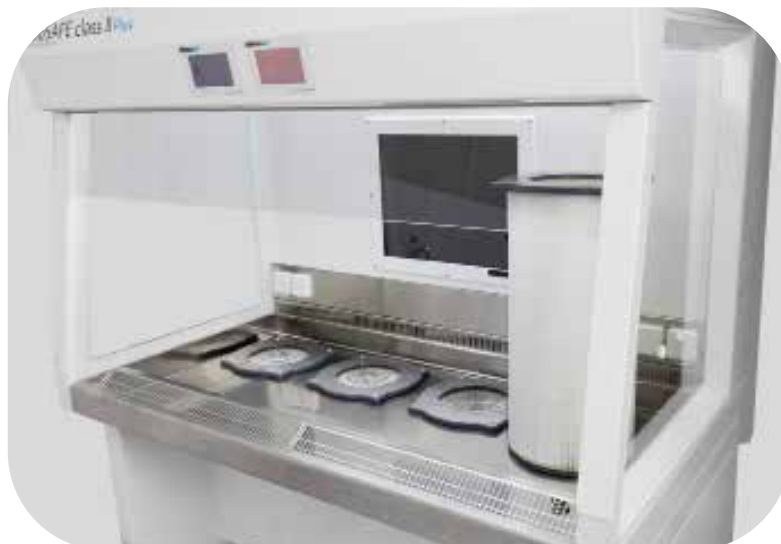
Optional H14 pre filters according to DIN12980
