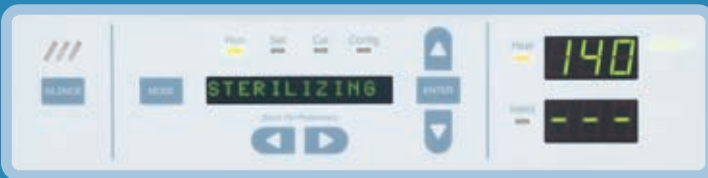
Sterilizing Phase – Chamber has reached the sterilization temperature and all microbial life is destroyed
