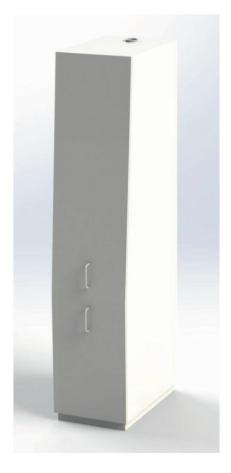
Ventilated chemical cabinet with split extendable front in the same shape as the fume cupboard 300x600x2000 mm (WxDxH) and 400x800x2000 mm. Chipboard frame with melamine laminate and drawer front in high-pressure laminate with stainless steel handle. 3 shelves in the upper part and 2 pcs. Shelves in the lower part.
