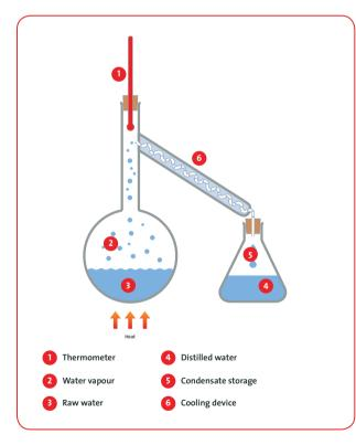
where cooling water lowers the temperature so that the water vapour is condensed, collected and stored. In principle, distillation can remove all classes of water contaminants, with the exception of those that have vapour pressures close to water and azeotropes. Distillation is most effectively performed with pre-treated water to minimise the build up of precipitates and the carryover of impurities.
