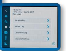
Internal data storage maintains a history of sample titrations, titrant standardizations, electrode calibrations and direct measurements – all with date and time stamp – to preserve critical data and facilitate easy data transfer to an external device.
