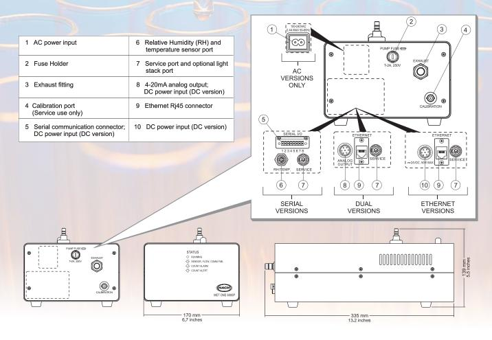
The MET ONE 6000P series remote airborne particle counter offers accurate and reliable continuous particle monitoring. With a sensitivity range of 0.5 to 10  $\mu$ m, the MET ONE 6000P series is designed to meet the specific needs of cleanroom operations within the pharmaceutical, semiconductor, hard disk drive and flat panel display industries.
